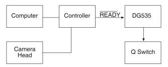
Figure 52. Setup using **READY** to trigger an Event
